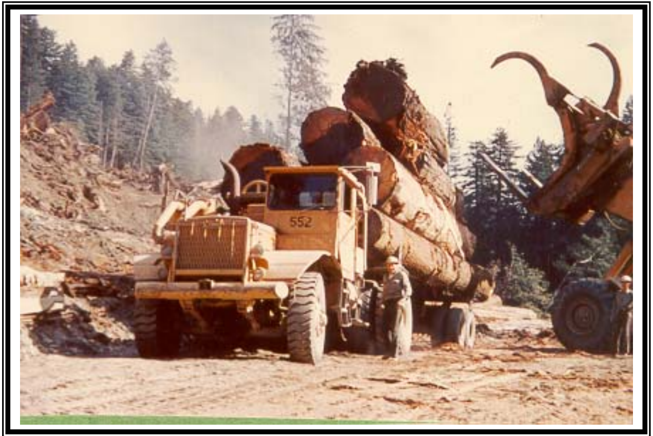
FRONTISPIECE: Thirty tons of truck ready to transport about 70 tons of Coast Redwood logs to the mill. On this truck the author rode and first viewed the bases for the conflicts that this book is about. Note two figures next to cab and far right for scale, and fact that the monstrous log loader at the right could be manipulated to turn a log a few inches as well as pick it up.
