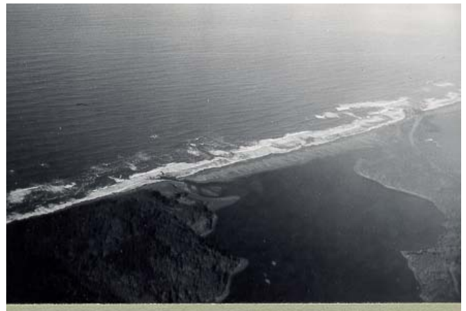
Figure 14 Flood flow has breached the sand and gravel bar that precluded flow from lagoon to sea.
